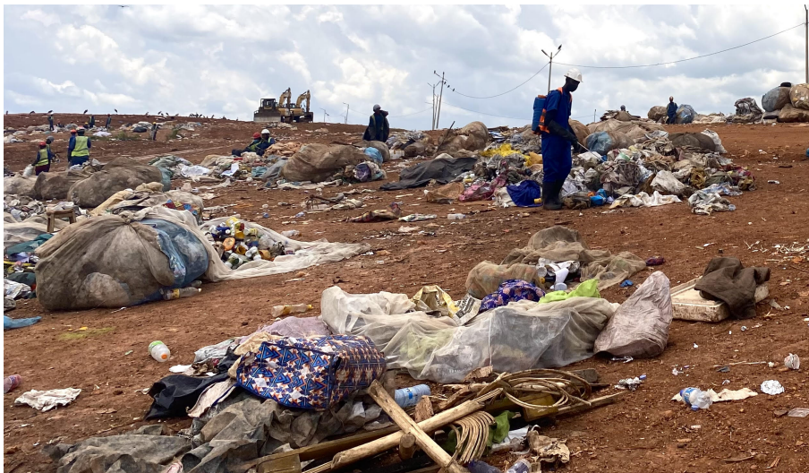
Figure 8: Manual chemical treatment on the received waste to prevent flies.
