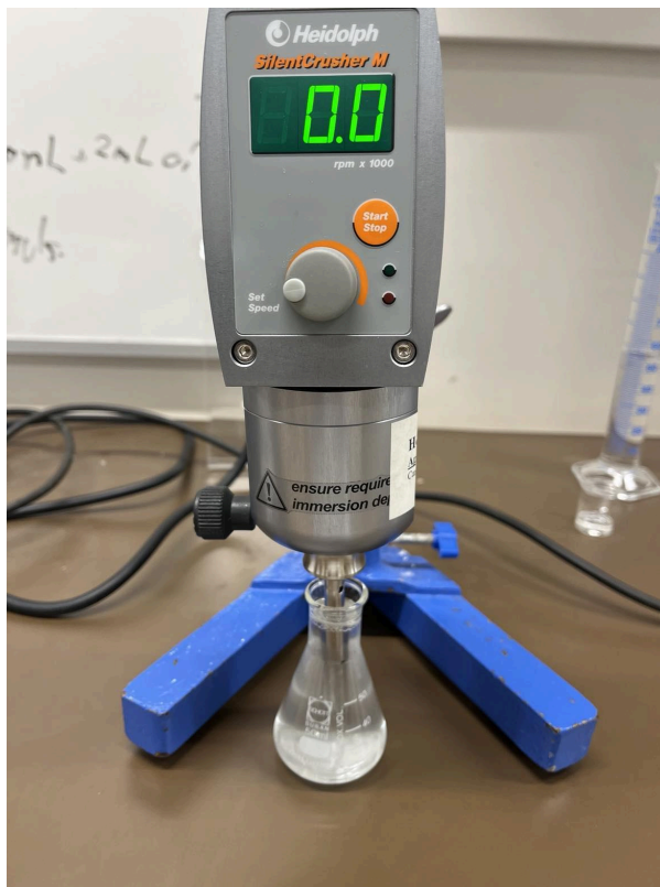
Figure 8. Shows the high shear mixer silentcrusher together with an erlenmeyer flask that is filled with distilled water, Pluronic F127, and miglyol oil.
