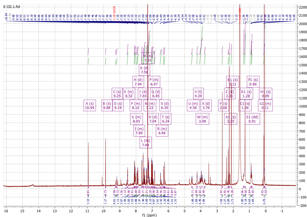
Figure 31, NMR for L3 in chloroform.
