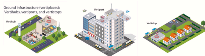
Figure 6. UAM infrastructure categories (Kiesewetter et al., 2023)
