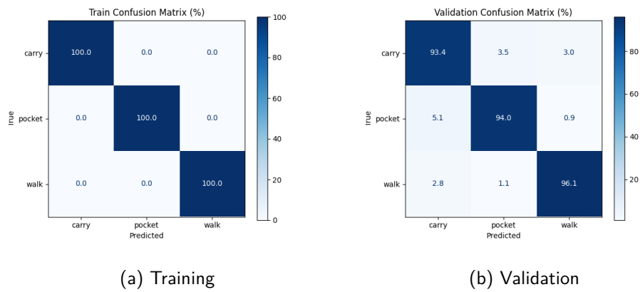
Figure 5.3: Confusion matrices for training and validation data using the Residual CNN model.
