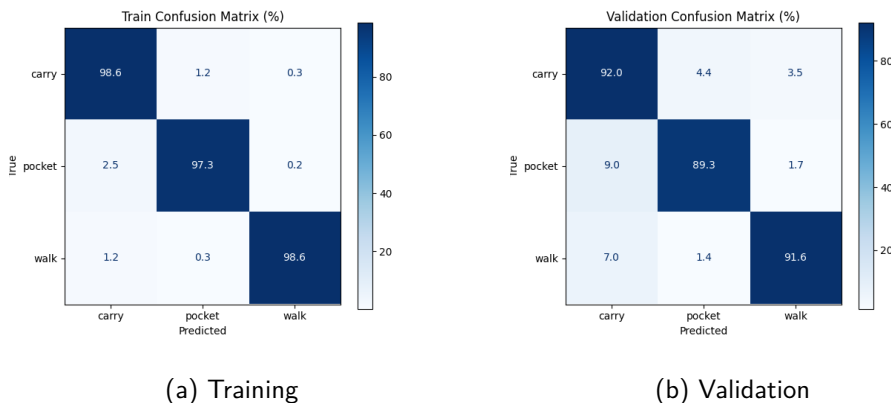
Figure 5.5: Confusion matrices for the CNN with attention model on the training and validation sets.
