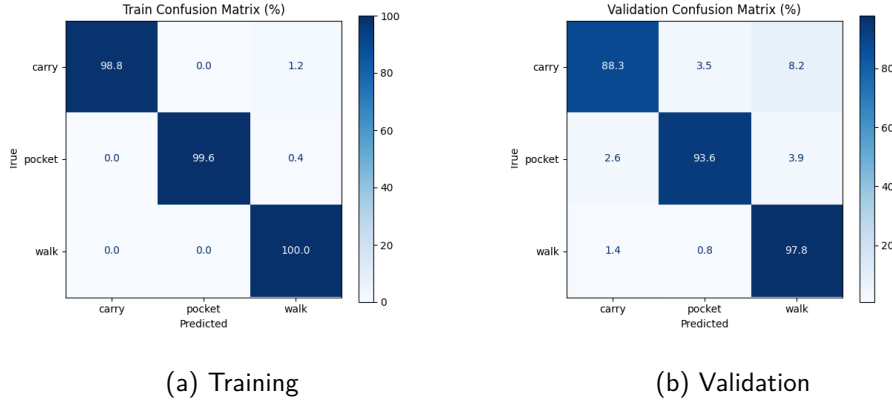
Figure 5.1: Confusion matrices for training and validation sets using the baseline CNN model.
