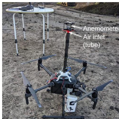
Figure 14: The setup of the UAV system by Gålfalk et al. (2021). The anemometer and air inlet marked with arrows are located 40 cm above the propellers.
