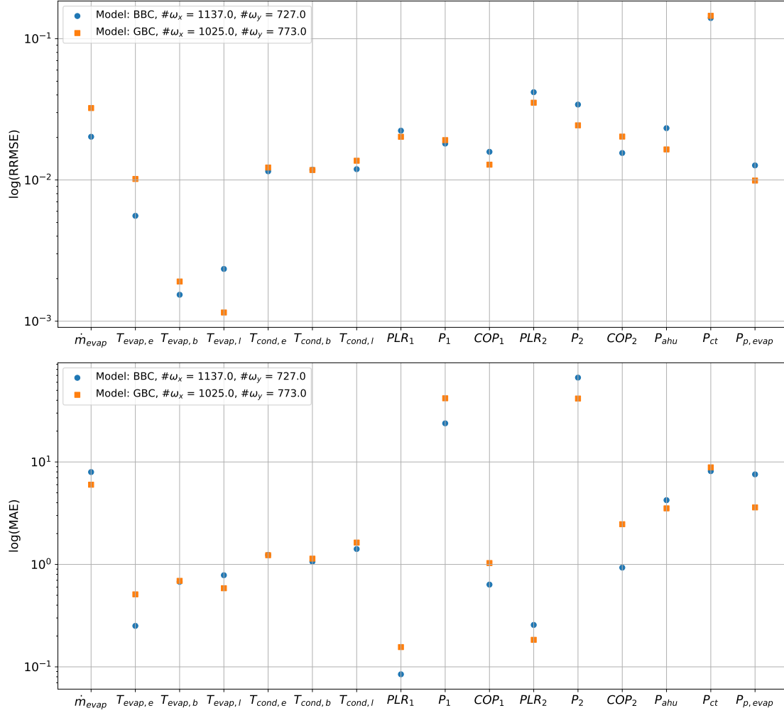
Figure 5.21: Comparison of Relative Root Mean Squared Error (top) and Maximum Absolute Error (bottom) across all predicted variables for the Black-box Component-Based and Gray-Box Component-based (GBC) approaches. The It load varied following a random step function in the training dataset and a constant function at 1.4 MW in the testing dataset.
