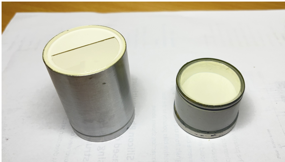
Figure 5: Two of the scintillators used in measurements. On the left is the irradiated \text{LaBr}_3 , and on the right the comparative \text{NaI}(\text{Tl})
