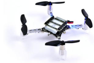
Figure 1. The Crazyflie 2.1 nano-quadrotor used in this project
