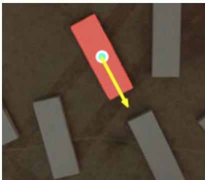
Figure 2. The binary mask in red, on a Jenga piece. The red represents the binary mask produced by SAM, the blue represents the estimated center of the block, and the yellow represents the orientation of the block.
