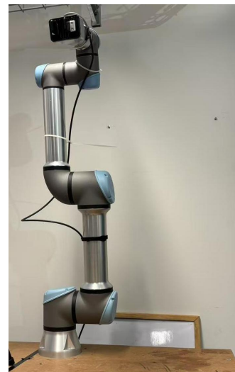
Figure 1. UR5e robot arm with gripper mounted, operating in the Jenga stacking environment.
