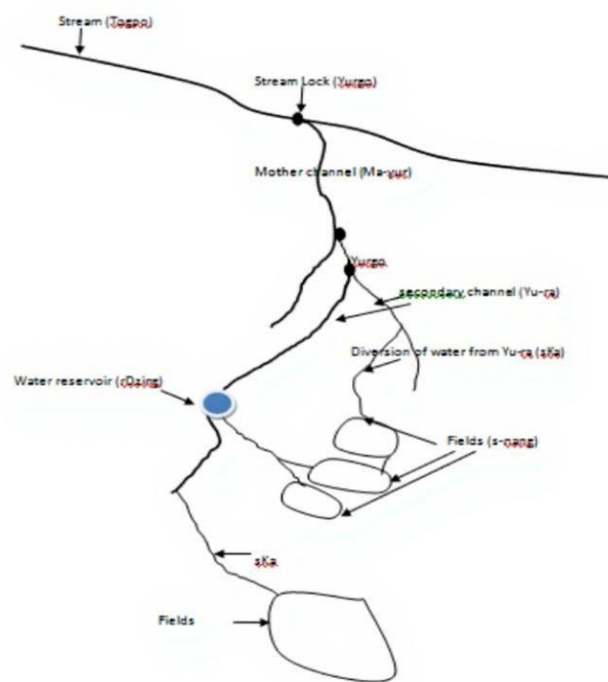
Fig.3: Schematic of water management system (Saxena, Raghuvanshi, et al., 2021)
