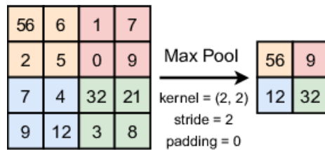
Figure 3: Example of a max pooling operation. Image courtesy of Shubhi Shukla et al.
