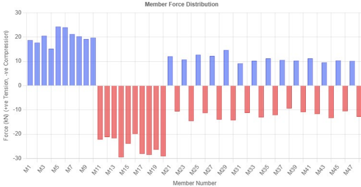
Figure 19 Force distribution of blue (tension) red (compression)
