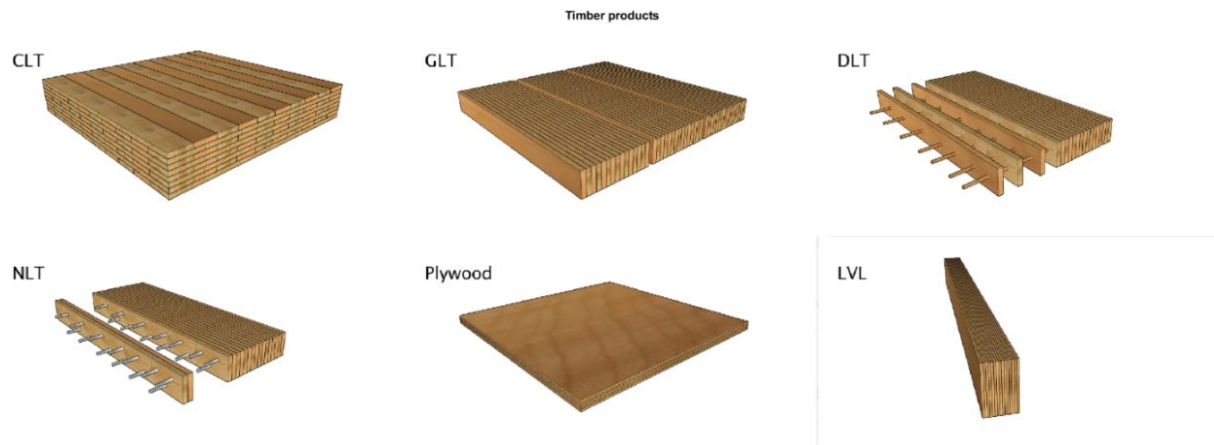
Figure 1 Different types of mass timber products. Adapted from Balasbaneh and Sher (2024); illustration by author.
