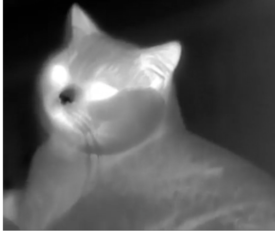
Figure 2.1: An example of a white-hot thermal image. Notice how the cat’s nose is the coldest part of the image, aside from the background.
