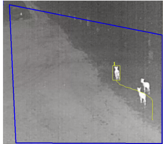
Figure 1.2: Here the initial deer has been detected but not yet classified, as indicated by its yellow bounding box. It has also been joined by two deer friends.
