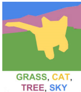
Figure 2.5: Semantic segmentation. Each pixel in the image is classified, resulting in the image being segmented into masks. [34].
