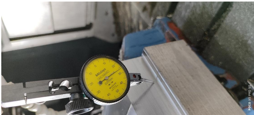
Fig 6.5 : Measurement of tool bending
