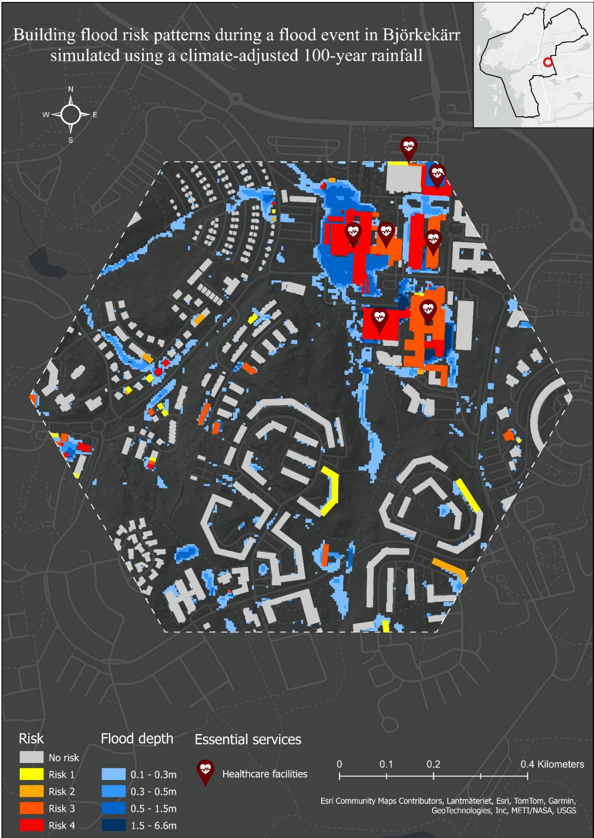
Figure 12. Spatial patterns of building flood risk in Björkekärr simulated using a climate-adjusted 100-year rainfall event.
