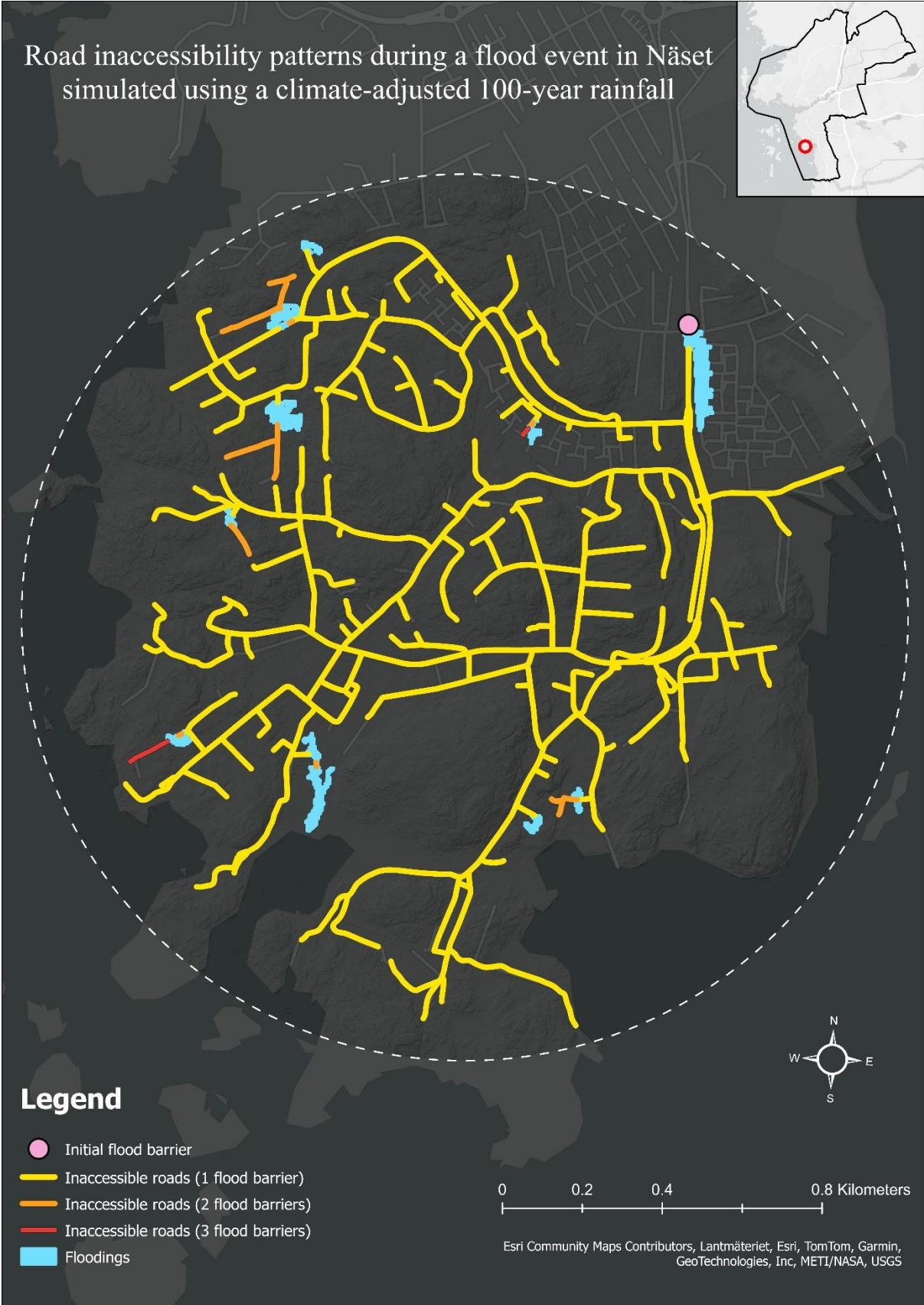
Figure 6. Spatial patterns of road inaccessibility in Näset simulated using a climate-adjusted 100-year rainfall event.
