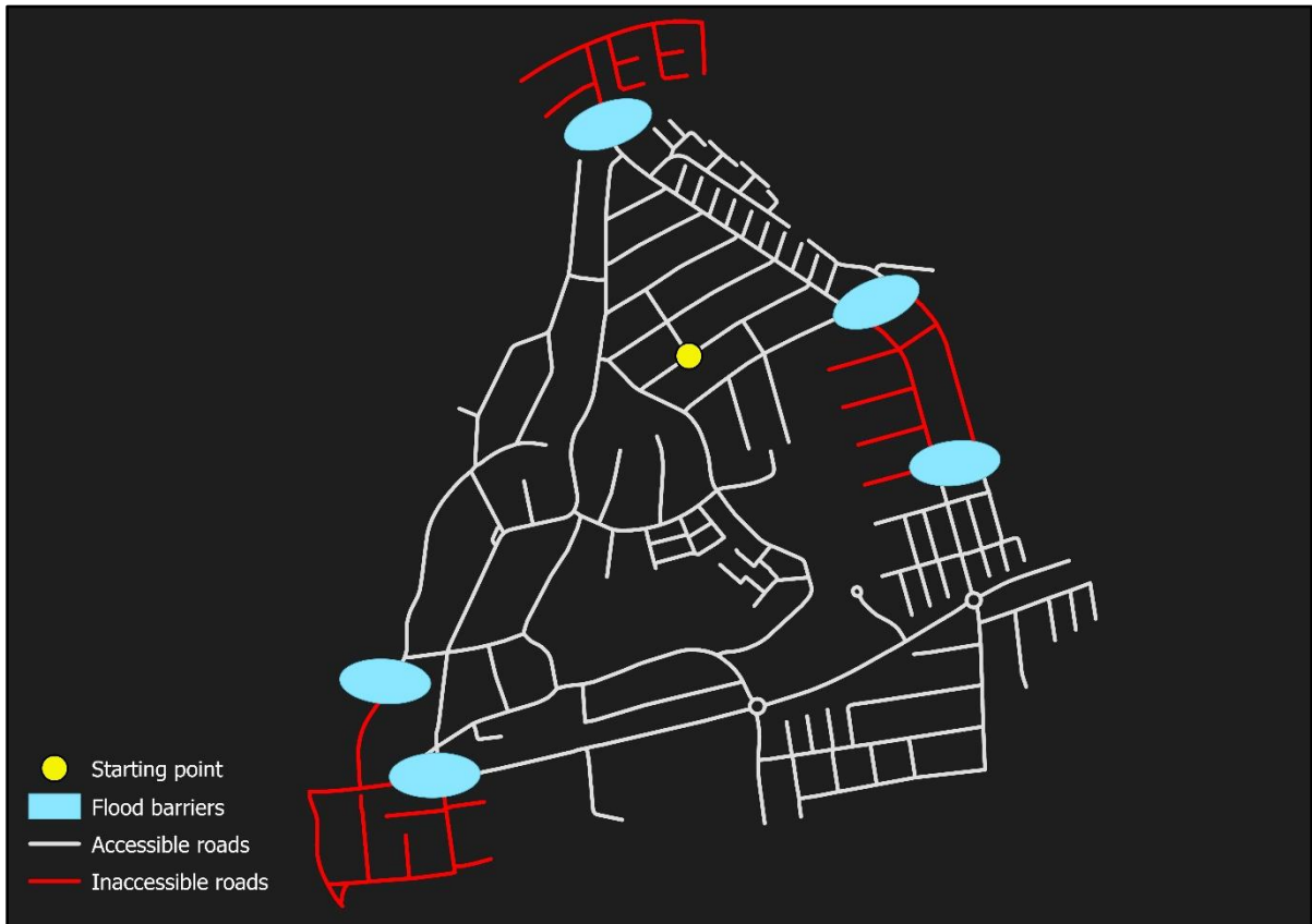
Figure 2. Illustration of the service area analysis used to determine accessible and inaccessible roads.
