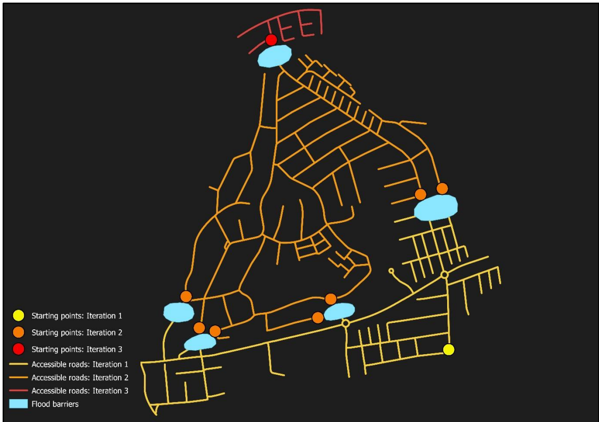
Figure 3. Illustration of the iterative service area approach for mapping road accessibility beyond flood barriers.
