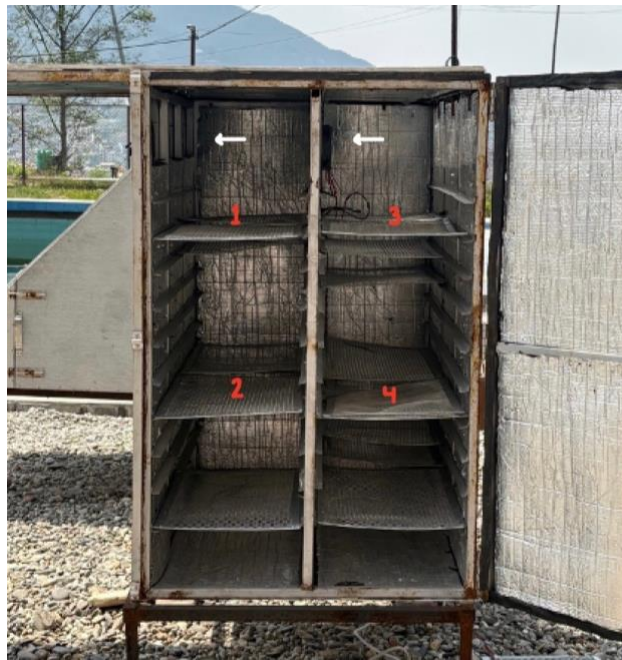
Figure 6: Inside of solar dryer, the red numbers (1-4) indicates where the dataloggers were placed in the dryer. The white arrows show the placement of the fans in the dryer.
