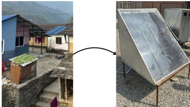
Figure 4.4: The SolarFood Project has created improved solar dryers (right) to help smallholder farmers transition from the less efficient open sun drying (right).
