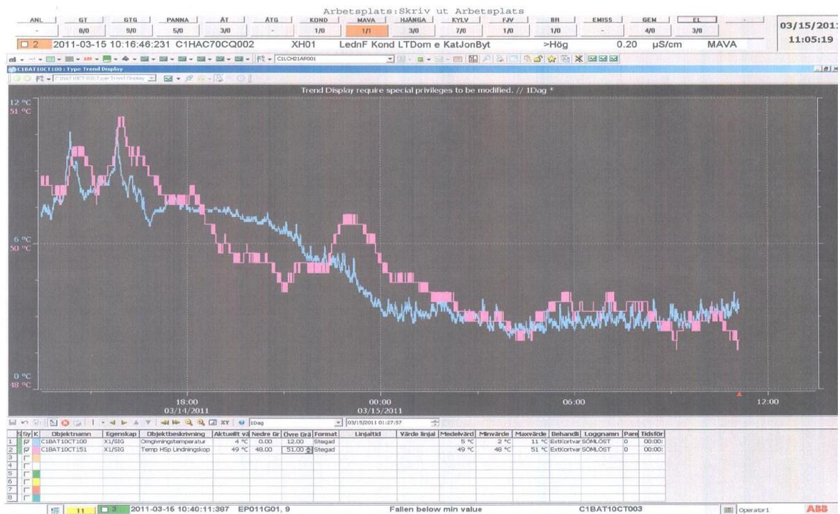
Graph 11.3: Windings oil temperature variations in manual mode (pink) of BAT 10 from 48°C to 51°C Vs. ambient temperature (blue) varying from 2°C to 11°C in 24 hours' time period.
