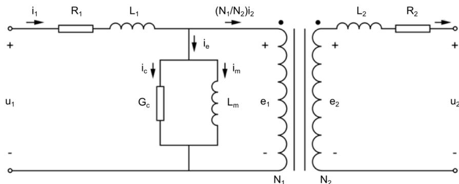
Figure 2.4: Schematic diagram of a real transformer [1]
