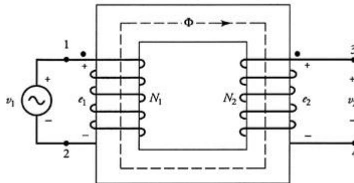
Figure 2.2 The single phase ideal transformer [1]
