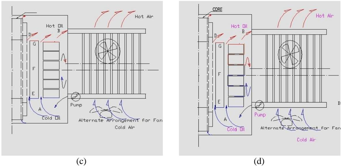
Figure 5.1 Oil flow diagram in ONAN(a), ONAF(b), OFAF(c) and ODAF(d) types of transformers.
