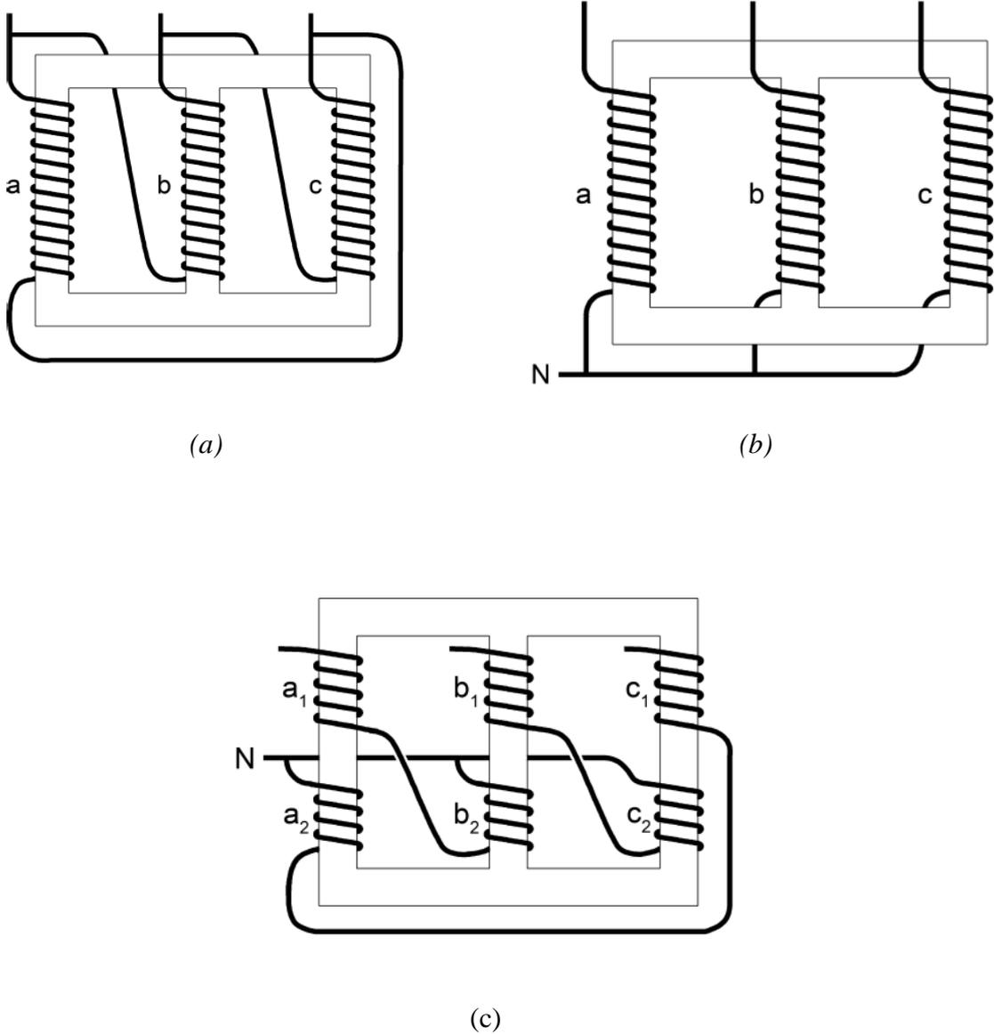
Figure 4.3 Delta (a), Y (b) and Z (c) connections [1]
