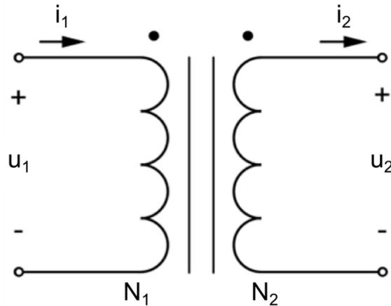
Figure 2.3 The circuit diagram of an ideal transformer [1]
