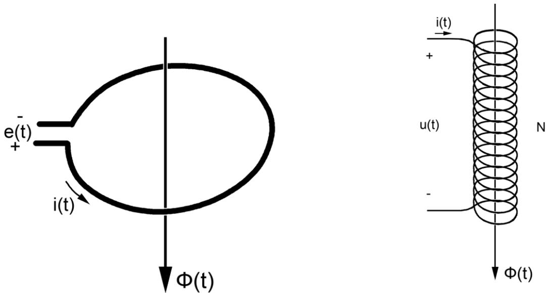
Figure 2.1 Direction of current and induced EMF in a coil with one and  $N$  turns in a magnetic flux [1]
