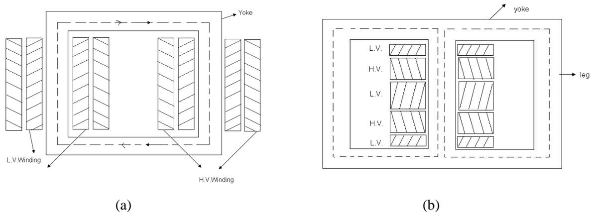
Figure 4.1 Core type transformer (a) and Shell type transformer (b)
