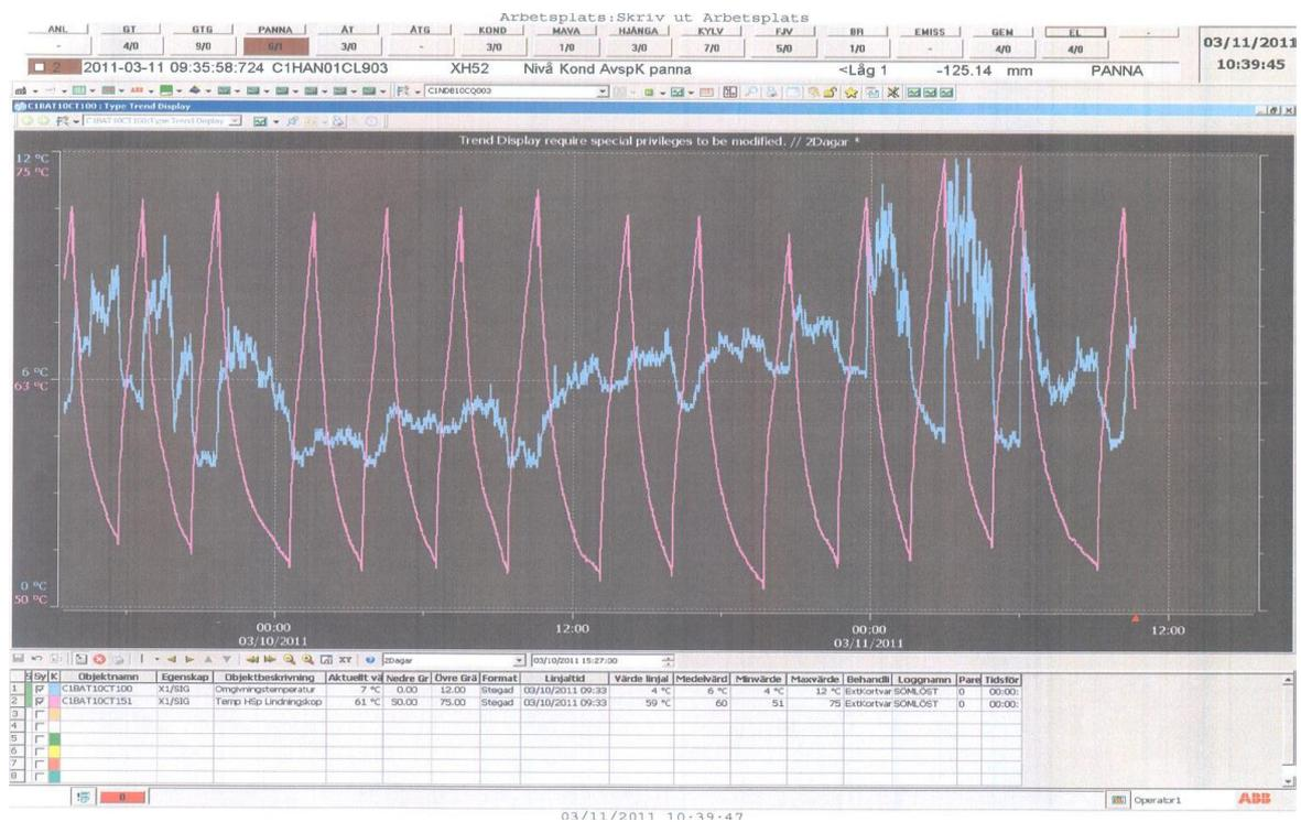
Graph 11.2: Windings oil temperature variations in auto mode (pink) of BAT 10 from 51°C to 75°C Vs. ambient temperature (blue) varying from 4°C to 12°C in 2 days' time period.
