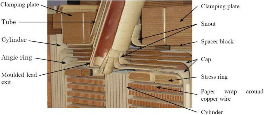
Figure 6.1: Cross-section view of a transformer end insulation [7]
