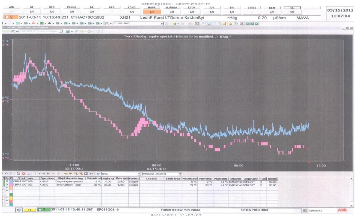
Graph 11.3: Top oil temperature variations in manual mode (pink) of BAT 10 from 38°C to 41°C Vs. ambient temperature (blue) varying from 2°C to 11°C in 24 hours' time period.
