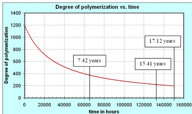
Figure 7.2: Degradation of DP value with time [7]
