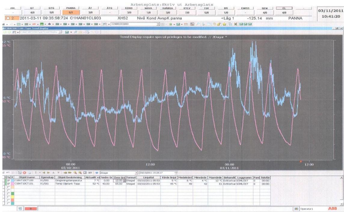
Graph 11.1: Top oil temperature variations in auto mode (pink) of BAT 10 from 49°C to 61°C Vs. ambient temperature (blue) varying from 4°C to 12°C in 2 days' time period.
