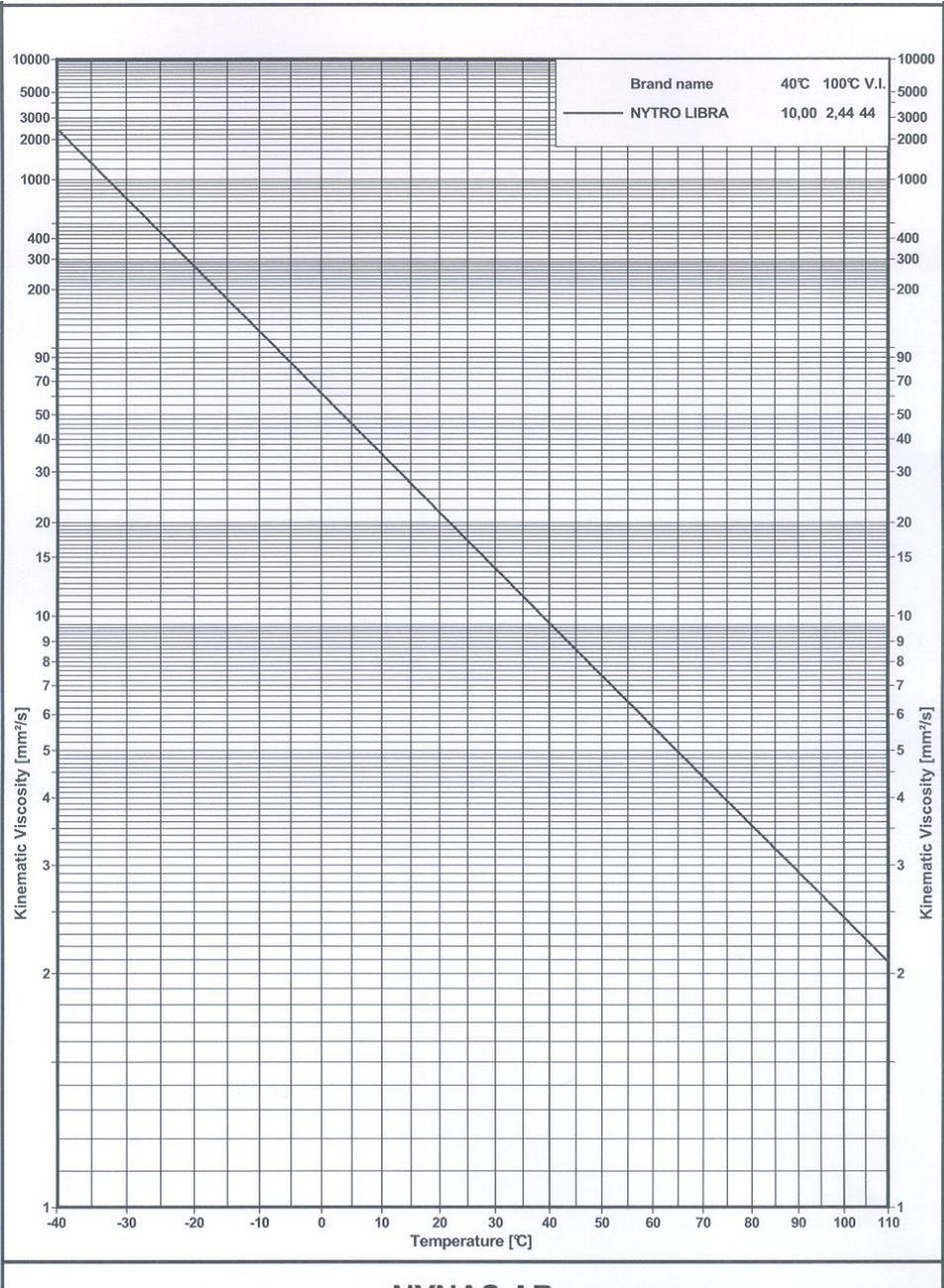
15.4 Inhibited Oil (Nytro 10XN) viscosity vs. temperature curve.
