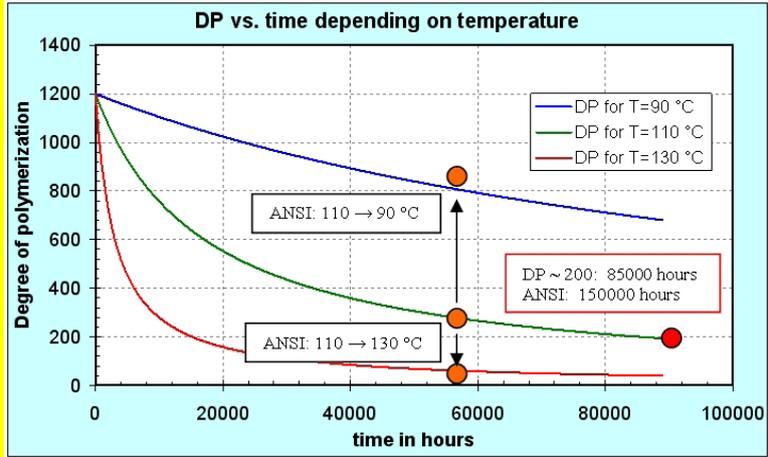
Figure 7.1 : Comparison between different DP values at different temperatures during the time. [7]
