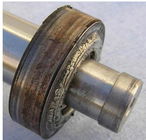
figure 29, bearing after two weeks of running
