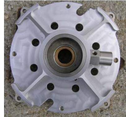
figure 8 , placement of the sensor at a bearing sleeve of a VA4111.
