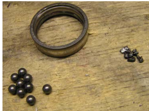
figure 39 , bearing parts. From left: ceramic balls, outer race and the rest of the cage.
