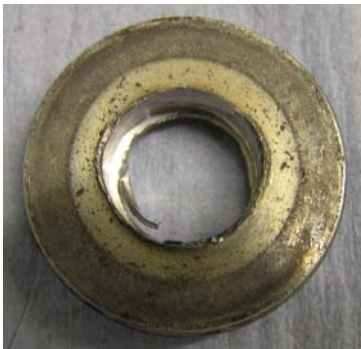
figure 38 , the emergency bearing sleeve. The tip of the rotor has enlarged the hole.
