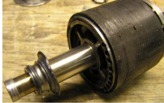
figure 37 , the rubbed rotor. Notice the rubbed tip. The bearing inner race and a protective plate are still attached.
