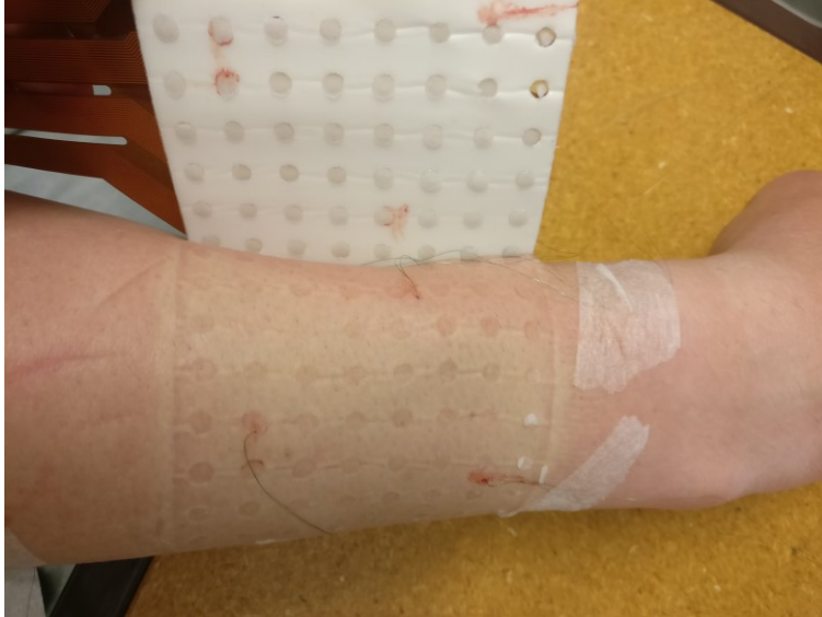
Figure 8. Image of the HDsEMG array and three iEMG wire electrodes on the subject's lower forearm.
