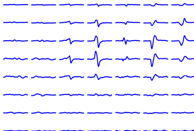
Figure 20. Extracted MU in the abductor pollicis longus muscle. Each sEMG signal was averaged using each instance of 184 firings in a MUAP train from HDsEMG decomposition. The far right column is excluded due to the nature of the differential recording setup. The trough in the fifth column is likely also due to the differential setup. The sixth column was used for depth estimation.
