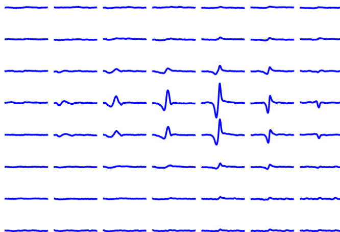
Figure 19. Extracted MU in the flexor digitorum profundus muscle. Each sEMG signal was averaged using each instance of 245 firings in a MUAP train from HDsEMG decomposition. The far right column is excluded due to the nature of the differential recording setup. The fifth column was used for depth estimation.
