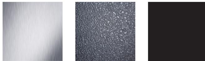
The material choices came natural, the body needed to be cast in aluminium to make it strong and using a rubber material on the top front to make it soft and comfortable when you raise. A rubber material would also be put on the bottom part of the support leg, to reduce the sound when the leg touches the floor.
