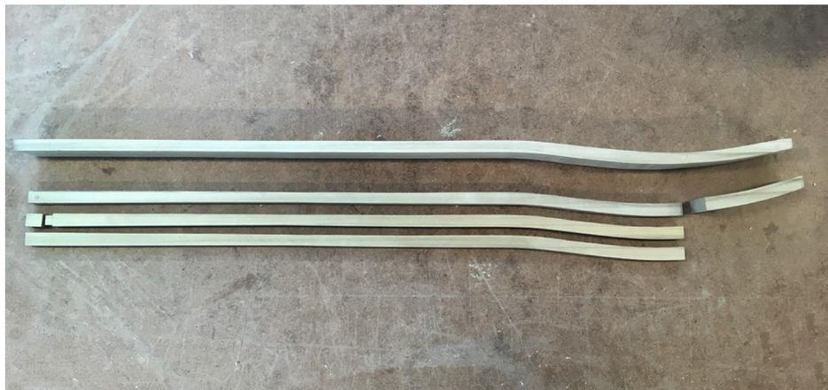
After making the technical drawing I went down to the workshop. To save money and time I decided to work with wood, poplar, for the prototype. I bought a solid piece of poplar and then sawed out every piece in the band saw. After this, I could easily sand the soft curves and make it super smooth. The sanding took a quite long time but it was something I had prepared for.
