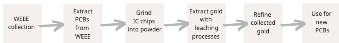
Figure 4-4. Dell’s Gold recycling process
