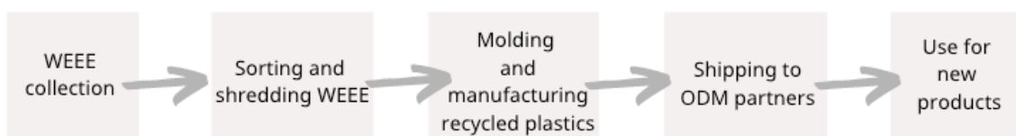
Figure 4-3. Dell's plastic recycling process
