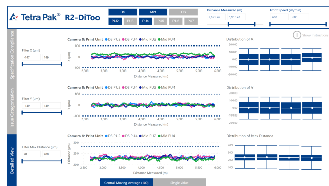
Figure 1. The R2-DiToo user interface, developed in Power BI, to visualize color-to-color register data from three inline cameras.
