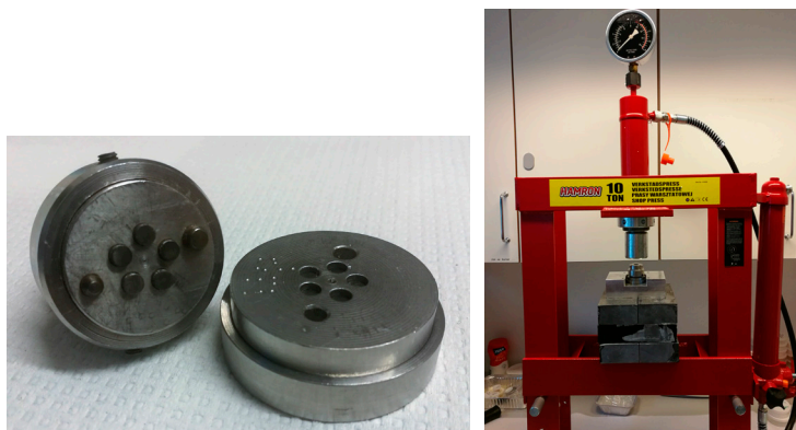
Figure 5. The in-house developed press tool (left) and the hydraulic hand press (right) used for making the pellets in Papers I-III.
