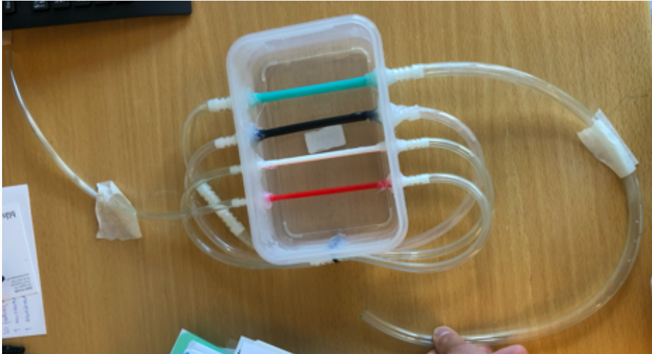
(a) Phantom with thin-walled vessels
