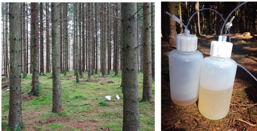
Figure 7 Spruce forest plot (61-years old; left) and lysimeter sampling bottles with soil solution (right) from Paper II.
