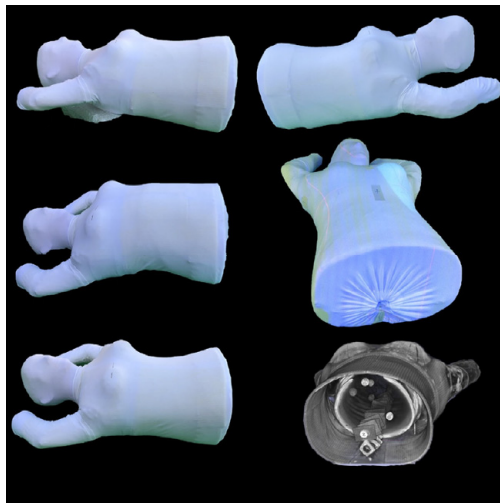
Figure 6. Anthropomorphic thorax phantom in different deformed positions, and a 3 dimensional model of the internal structures used for cone beam computed tomography verification.
