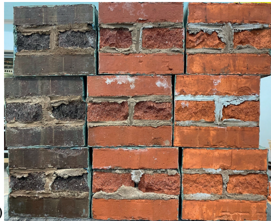
Figure 13. a) Representative specimens from each group and Series after sealing; b) Schematic of the mortar joint profile finishes, and c) Backside of representative specimens
