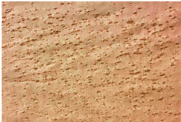
Figure 10. Wet dots on a paper sheet exposed to water spray for 1–2 seconds.
