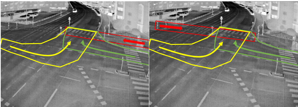
FIGURE 8: The goal is to find times when a vulnerable road user is moving through the red regions in the marked directions, while a car is moving either through the green or yellow regions simultaneously.
