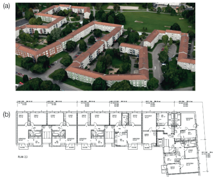
Figure 3.8 a) Aerial view and b) typical floor plan for a part of a “semi-open courtyard” development. Multiple parts of this development were included in the simulation study. Notice the narrow building volume (8.9 m wide), with two apartment units per stairwell across the linear part and three units in the part that forms the courtyard corner. Figure 3.8a © Google. Figure 3.8b was retrieved from the municipal drawing archives of Stockholm (“Stockholm stad, Bygg och plantjänsten (In English: Stockholm city, Construction and planning service),” 2018).
