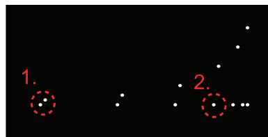
Fig. 1. Ultrasound phantom structure. Dashed, red circles mark areas where individual RF data lines were analyzed.
