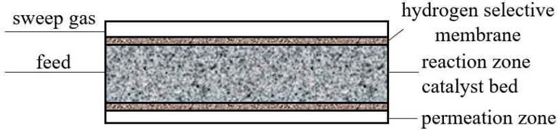
Figure 2.6: Hydrogene selective membrane reactor schematic.
