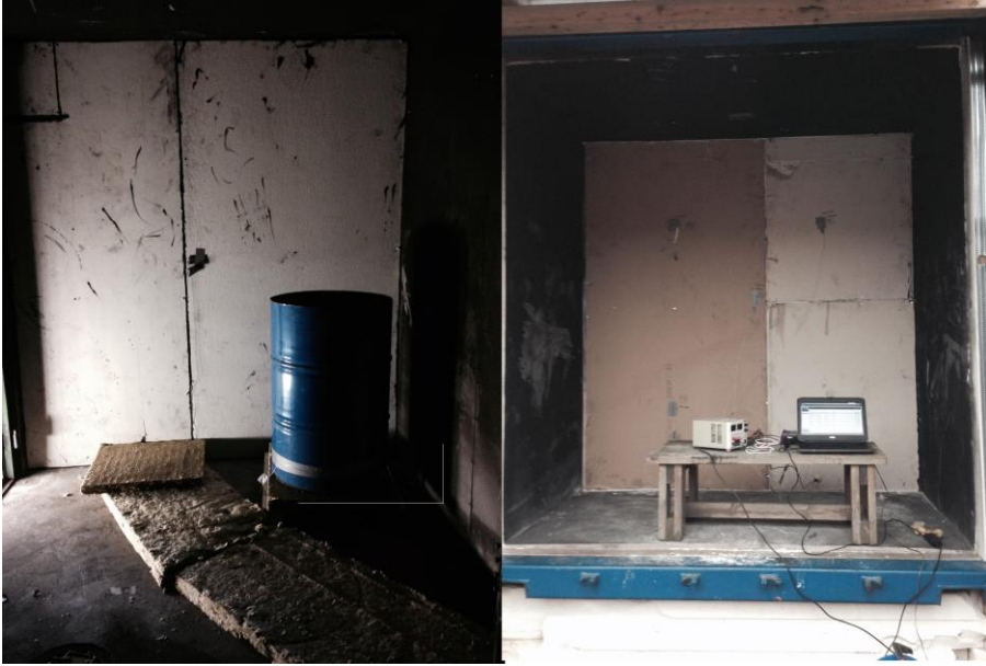
Figure 24: Experimental set-up for the compartment fire.
