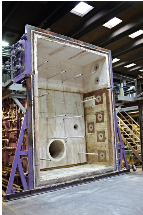
Figure 5: Image of a Standard Fire Resistance Vertical Furnace at DBI (Copyright: The Danish Institute of Fire and Security Technology)
