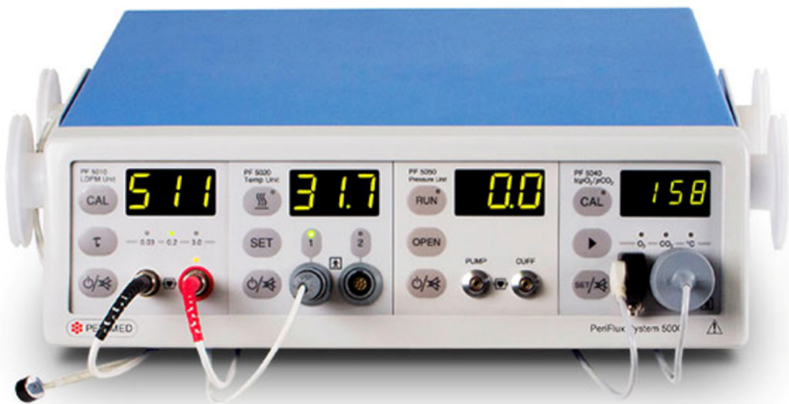
Figure 9. Showing the Laser-Doppler velocimetry machine. Reprinted with the permission from Perimed AB.
