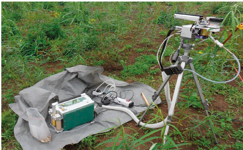
Figure S1. Experimental setup of leaf chamber system. To the right on the top of the tripod, the leaf chamber is attached and connected to the portable photosynthesis system (LI-6400) to the left. BVOC-sampling was done by taking a sub-sample of 200 ml/min of air leaving the leaf chamber using adsorbent tubes filled with Tenax TA and Carboxograph with a small flow regulated pump.
