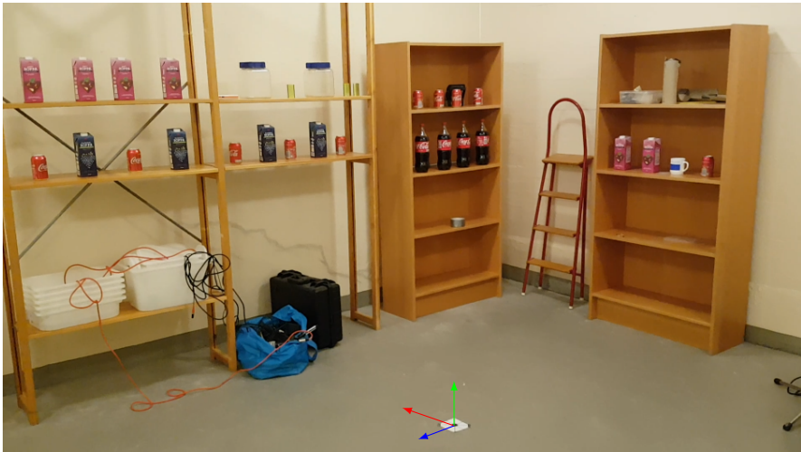
Figure 4.8 Depiction of the setup in which the second example is run. A set of shelves with various drinks are to be scanned, with the camera facing the target shelf at all times. The origin of \{\mathcal{G}\} is defined on a piece of paper.
