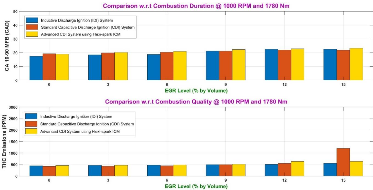
Figure 30: Comparison of Combustion Quality and Main Combustion Duration @ 1000 RPM and 1780 Nm
