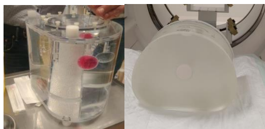
Fig. 2. NEMA-IEC phantom design.
