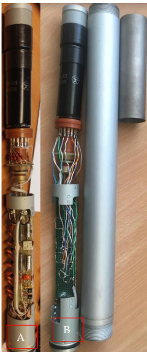
Fig. 8. A - \phi_{3y} - 85 PMT with initial circuitry; B - with new voltage divider and used shielding
