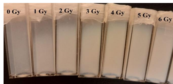
Fig. 1. Improved NIPAM polymer gel dosimeter samples fabricated using "hot" procedure and irradiated with doses from 1 to 6 Gy.
