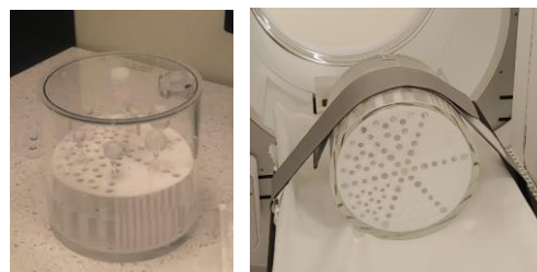
Fig. 1. Jaszczak phantom with inner structures.
