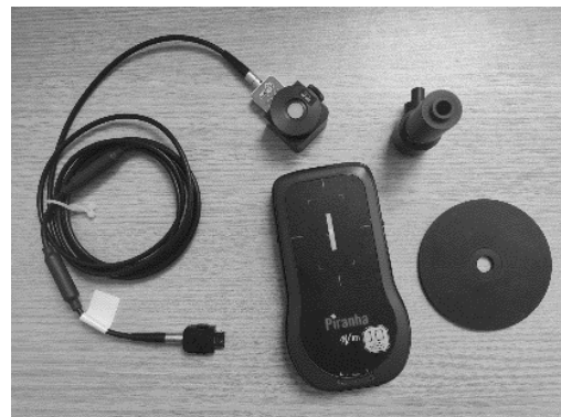
Fig. 1. Piranha RTI 657 with LightProbe L100 sensor and its attachments.
