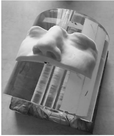
Fig. 1. The printed phantom is attached to the surface of the PMMA CT Head phantom
