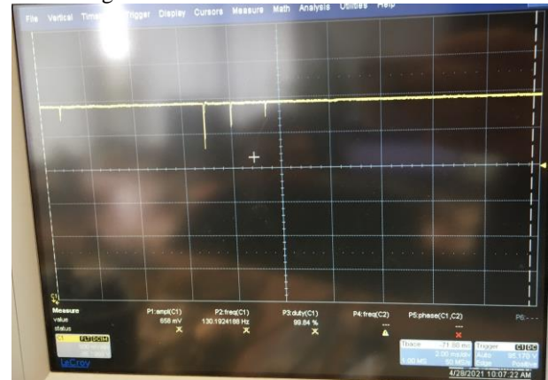
Fig. 9. Clean pulses from PMT when powered from GS-USB-PRO
