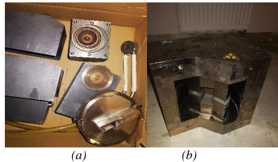
Fig.3 Activated linac parts, vacuum window of the accelerating wave-guide, the target and the flattening filter (a), bending magnet core (b)
