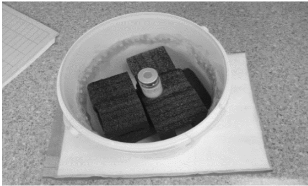
Fig. 1. Calibration of TLD-100 chips with ^{99m}\text{Tc} source.
