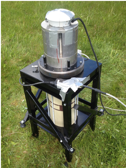
Figure 3.11: The collimator system as used in the tests. The GPS antenna is placed on top of the collimator. The slit opening, showing the HPGe detector, points towards the camera. The stand supports the detector and the rotation mechanism that in turn holds the collimator. The liquid nitrogen Dewar for the HPGe detector can be seen in the middle of the stand. The electronics are outside the field of view of the camera.
