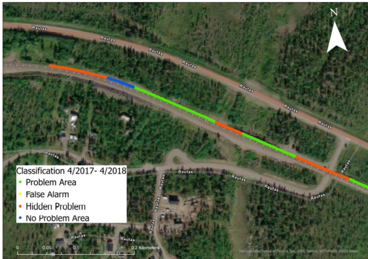
Figure 15. Example of a Classification of InSAR-based and Optram-derived Changes
