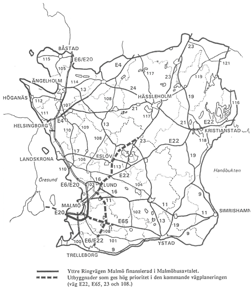
Figure A.2 road investments in the Malmöhus Agreement. The thick solid line indicates the ring road around Malmö, that was the only part financed in the Agreement. Dotted lines indicate projects not included in the agreement to be prioritized in coming road plans. Source: SOU 1992:114 , 20.
