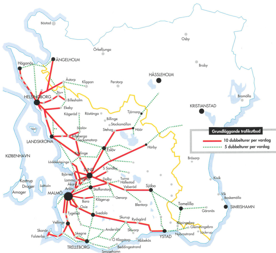
Figure 9.3 Map showing traffic supply frequency in Malmöhus in 1998. Solid lines are relations with 10 reutrns trips daily, broken lines show relations with 5 return trips. Source: Malmöhus Trafik: Som på räls . 1998, 17
