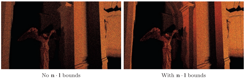
Figure 18-10. Visual results when not using the \mathbf{n} \cdot \mathbf{l} bounds (left) compared to using it (right). Both images use 8 SPP (4 BRDF samples and 4 light samples) and a BVH binned along all three axes with 16 bins using SAH, and both take into account the distance and flux of the light.
