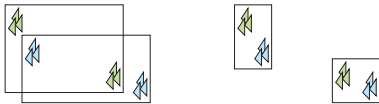
Figure 2: Care has to be taken when deciding which light sources to put in each bottom-level hierarchy. Left: it is difficult to accurately estimate the contribution from the large overlapping BLASes, leading to higher variance. Right: it is preferable to place lights that are spatially nearby in the same hierarchies.
