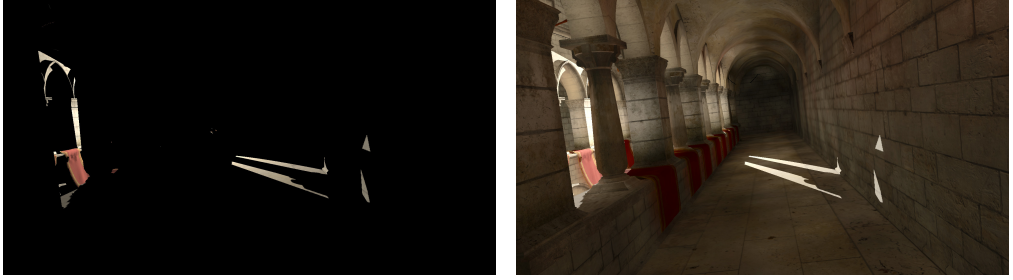
Figure 10: Visualising the impact of indirect illumination in certain scenarios. On the left, only direct lighting is present, while both direct and indirect are computed in the image on the right. The renderings were taken from the author’s master thesis. The Sponza scene was created by Frank Meinel and is available under the CC-BY-3.0 license from Morgan McGuire’s Computer Graphics Archive [32].
