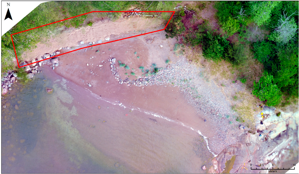
Figure 4-5. Aerial photograph of the embayment at Nykvarnsholme. The photo was taken one month after nourishing the bluff (red area). (Photo by Mats Öberg, SGI)
