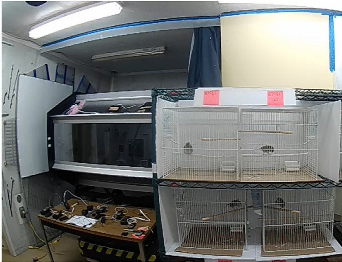
FIGURE 1 | Experimental caging in the wind tunnel plenum. Sparrows were held individually in cages on racks adjacent to the working (flight) section of the wind tunnel that can be observed to the left. A baffle (white panel) ensured air mixing between the plenum and working section so that temperature, humidity, and pressure in the plenum was identical to the air flow in the tunnel.
