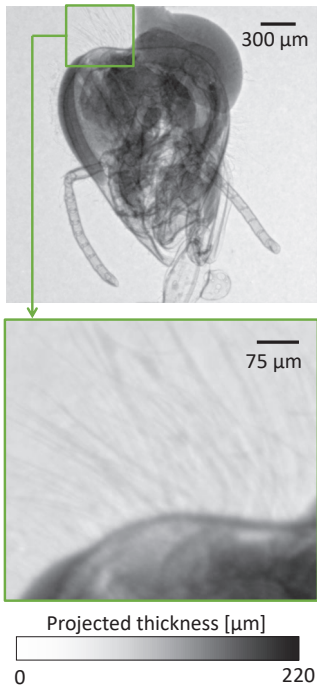
Figure 4.19. Projected thickness, \Gamma(\mathbf{r}) , calculated using Equation 4.15. The sample is the head of a bee which was glued onto a needle. Some of the glue is visible in the upper right part of the image.
