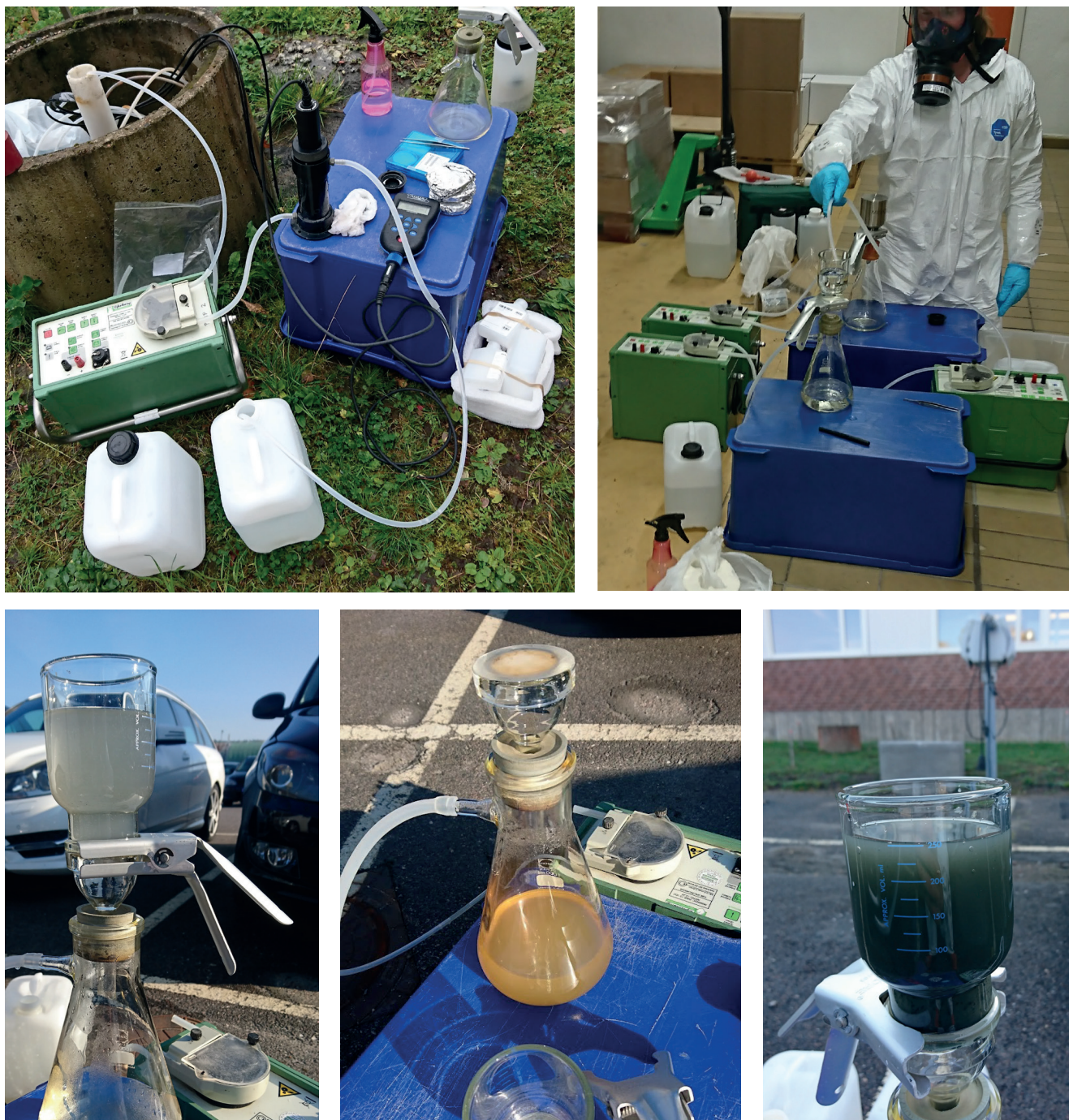
Figure 9. Photos from fieldwork in Alingsås. A) The set-up for the pre-purge process in combination with monitoring of physical properties. B) The sampling set-up during microbial sampling. C) Filtering water from MW4 in 2018, grey colored. D) MW4 with filtered water, rust colored likely due to oxidation of iron coming from Area A. E) Filtering water from Area B in 2018, a thick and dark liquid.
