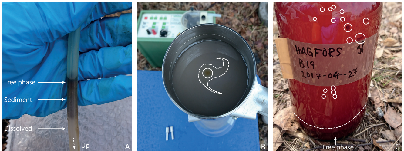
Figure 3. Photos from the field work, seeing CAH in free-phase at the first field site (Hagfors), where CAH for unknown reasons is colored dark. A) The tube turned upside down, with free-phase product at the bottom, sediment and dissolved contaminants. B) A “bubble” of PCE marked with the circle and dissolved halo. C) “Bubbles” of free-phase sinking in the bottles (circles) towards the bottom marked with a line.
