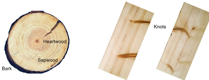
Figure 2.1. To the left, the cross-section of a Scots pine stem with the darker heartwood surrounded by lighter sapwood and outermost the bark. To the right, boards of Scots pine (left) and Norway spruce (right) with knots visible as darker patches.
