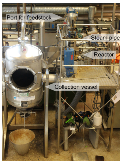
Figure 3.9. The biomass was pretreated by steam explosion in batches of typically 600-700 g of dry matter in a 10 L reactor described by Bondesson et al. (2014).
