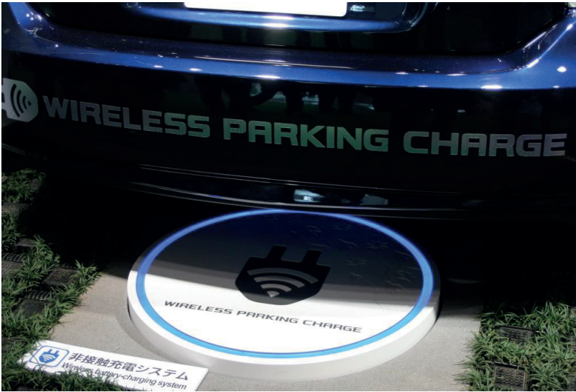
Figure 1.4: An inductive charging pad [14].
