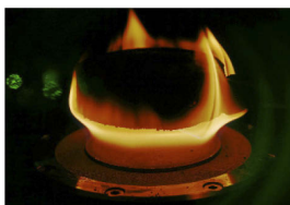
Fig. 3. Luminous ethylene/air flame at equivalence ratio \Phi=2.0 . The flame photo was taken through a 532 nm notch filter to block strong green light from the laser, and the brightness-contrast level has been adjusted to make the burner visible.
